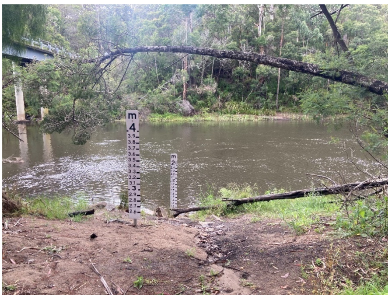
Figure 4: Bemm River Gauge boards installed at Old Coast Road
